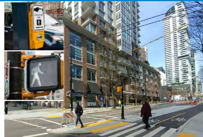
Curb ramps between sidewalk and street + Tactile walking surfaces for directional guidance + Accessible pedestrian signals (Richards St, Vancouver)
