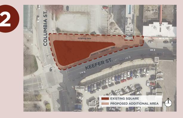
This idea expands the square into the existing road space while maintaining existing traffic circulation and site access. The increase in space would be achieved by reducing lane widths, shifting lanes and moving curbs. This results in an increase of 900m<sup>2</sup> (approx. 130%). The main considerations for this idea include:
