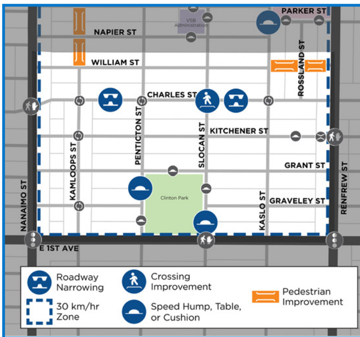
Figure 10. Proposed Zone 2 (South) vehicle speed reduction & safety measures
