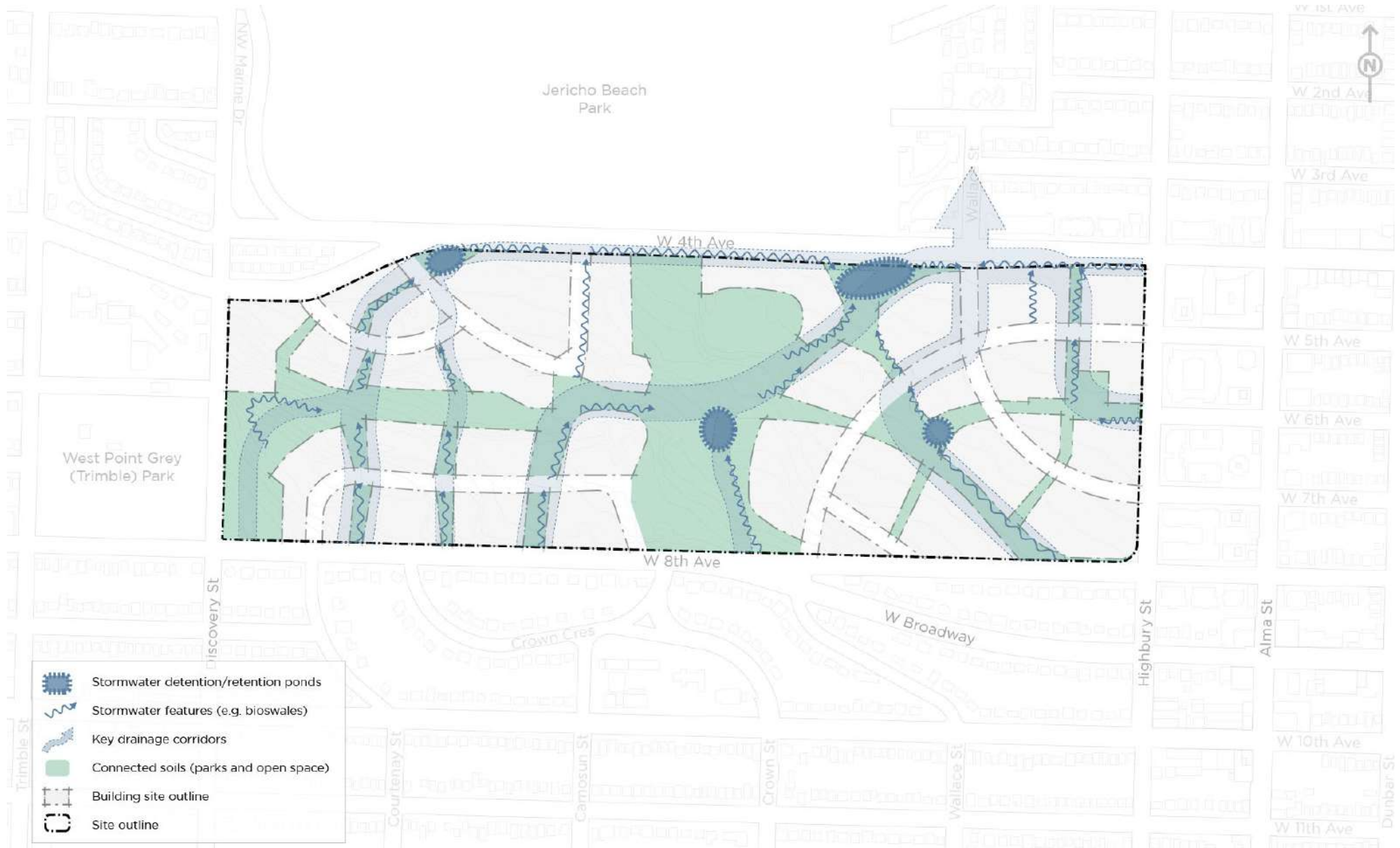
Figure 8: Water Management and Key Drainage Corridors
