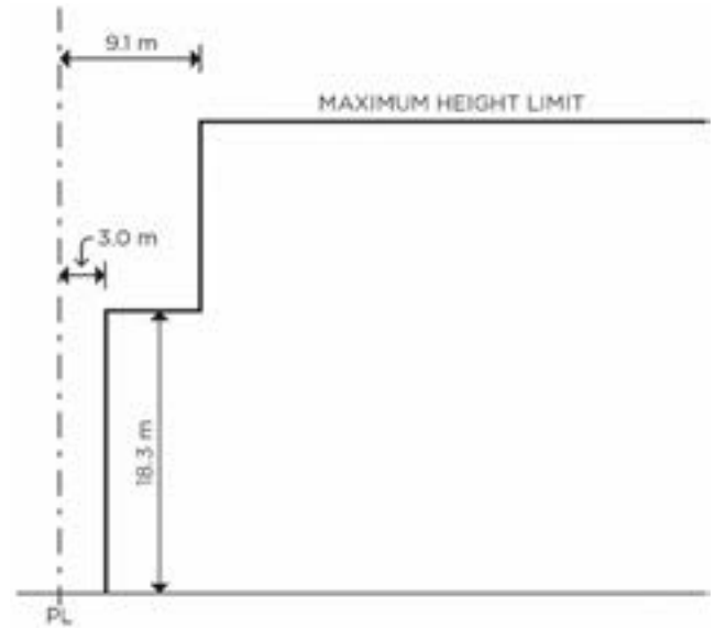
Diagram: Building Height Limit at North-South Lane between 2nd Avenue and 5th Avenue
