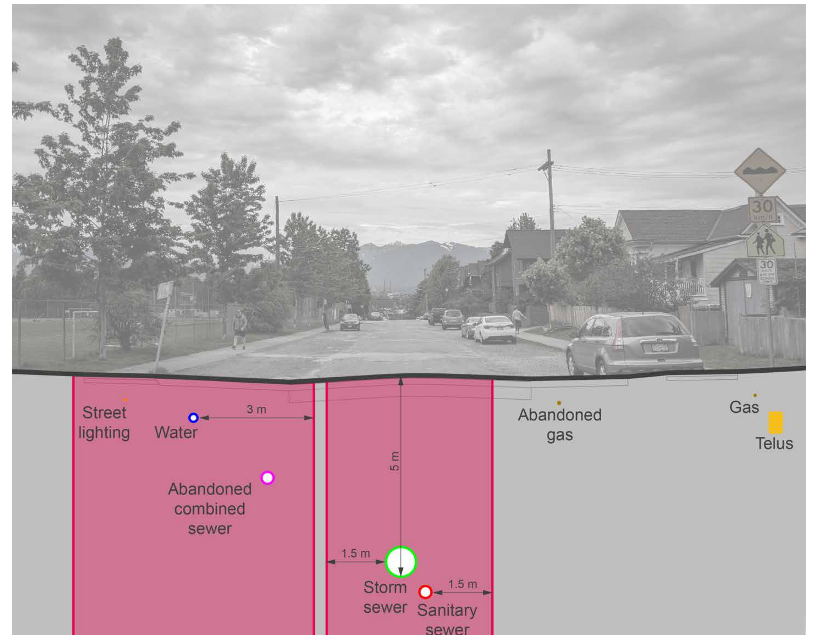
This diagram of St. George Street highlights both the required utility setbacks, as well as the depth at which the lost stream is buried.
